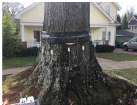
Arbotom tool being used to inspect a large oak on Euclid Ave. Photo courtesy Tim Porter.
